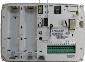
\* When using the XTIP panel with the Ethernet connection or SMS Arming you must use a 12v 2A Power Supply with 4 Alkaline battery backup (PP4)\*
